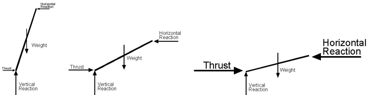
a typical rafter can be significant. For instance, on a typical 6:12 roof on a 30-foot wide house, the thrust at the base of each rafter is 700#. For a 3:12 roof, the thrust is 1400#.
