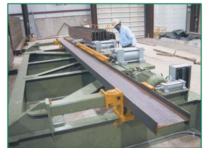
Photo of beam cold cambering.
